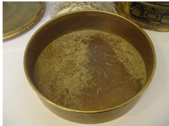
Figure 12. Bottom tray collects the remaining fine particles
