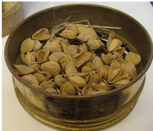
Figure 7. Sieve-1 (opening 18.850mm) contains mostly nuts and twigs
