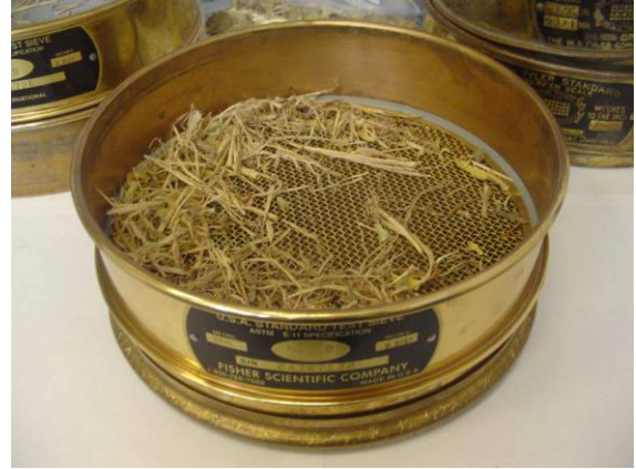
Figure 10. Sieve-4 (mesh #10, opening 2mm) contains mostly grass
