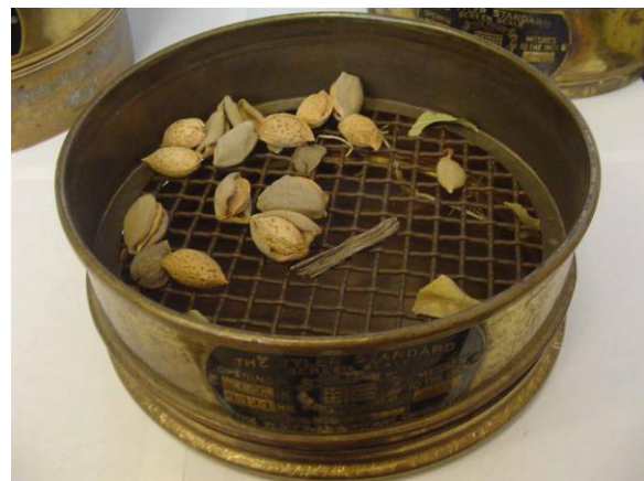
Figure 8. Sieve-2 (opening 9.423mm) contains small nuts, leaves, and small twigs
