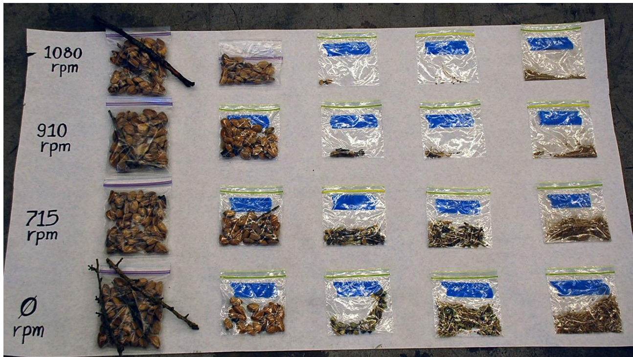
Figure 13. Sieve analysis of example replicate (1) windrow samples from Arbutle on August 18 th -19 th 2008. From left to right: particle size \geq 18.850 mm, 9.423 mm \leq particle size \leq 18.850 mm, 5.6 mm \leq particle size \leq 9.423 mm, 2 mm \leq particle size \leq 5.6 mm, particle size \leq 2 mm.
