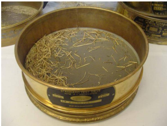
Figure 11. Sieve-5 (mesh #20, opening 0.850mm) contains mostly grass.
