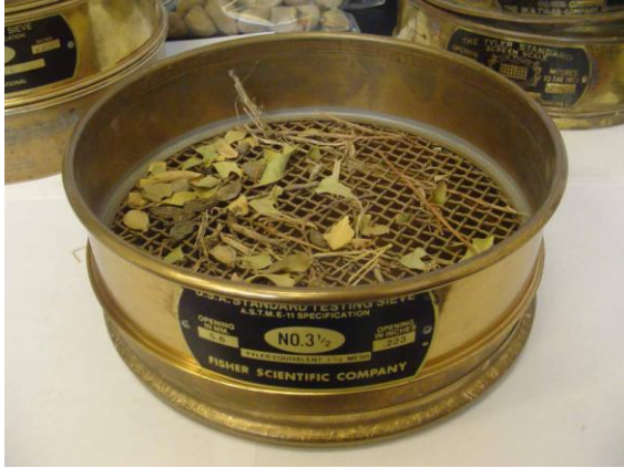
Figure 9. Sieve-3 (mesh #3.5, opening 5.6mm) contains mostly leaves and grass
