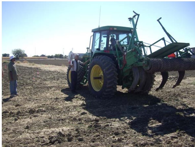
Figure 2b: TriCal Shank type fumigant applicator retrofitted with a planting-site specific fumigant application system.
