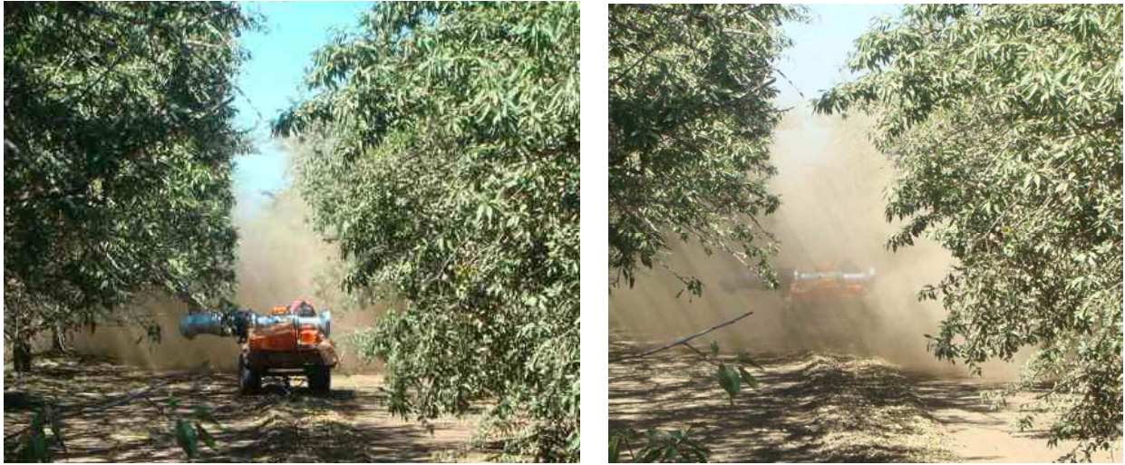
Figure 2. Approach of harvester to the opacity sampler (left image) and harvester discharge plume sampled by instrument (right image). In both cases harvester is in row to right of sampler.
