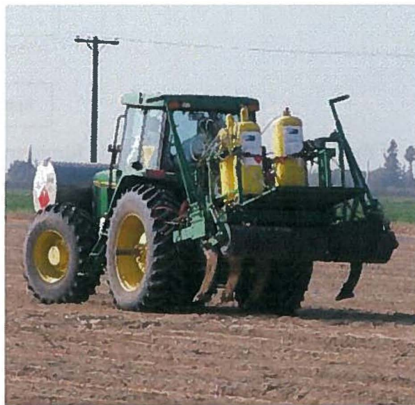
Figure 1. TriCal fumigation tractor with subsoiler shanks.
