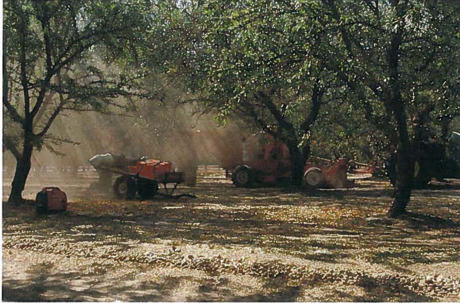
Figure 2. Stationary opacity measurements and portable air samplers positioned within the orchard during harvester test runs.
