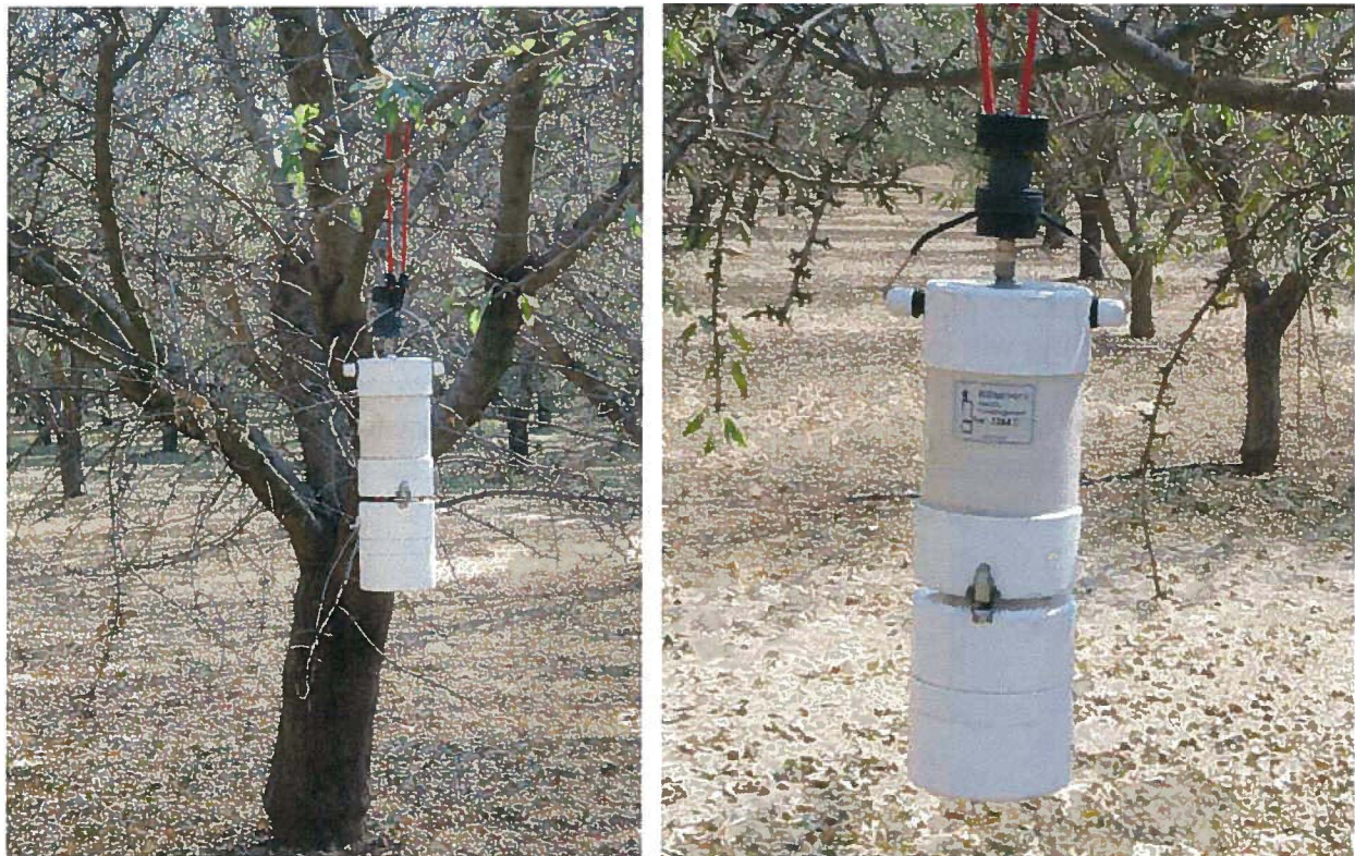
Figure 1. Portable air samplers positioned within the orchard during sweeping and harvester test runs.
