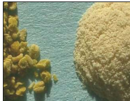
Figure 2. Magnified image of unwashed Nonpareil pollen (left) compared to washed and filtered pollen (right).
