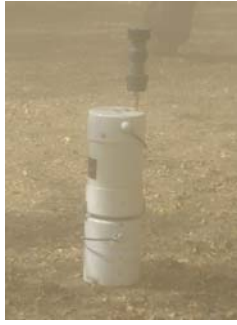
Figure 1. MiniVol™ sampler with PM2.5 inlet located within the dust plume one row away from harvest row.
