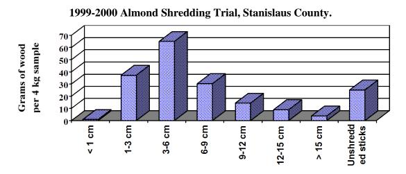
*Fig. 1.* Woody debris in nut cart samples at harvest segregated by length. Prunings were shredded the previous fall with one pass of a tractor-mounted brush shredder.
