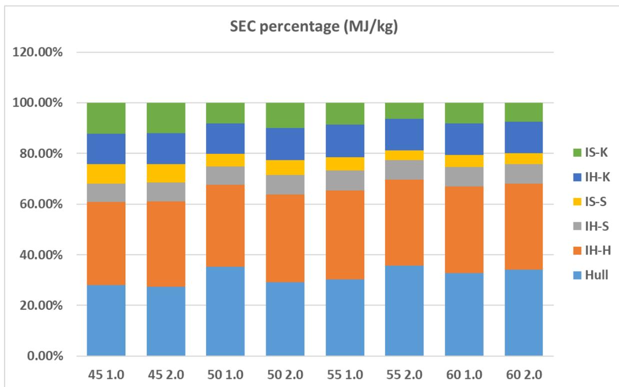
Figure AB.43 Specific energy consumption (SEC) for column dryer at different drying conditions (NP)
