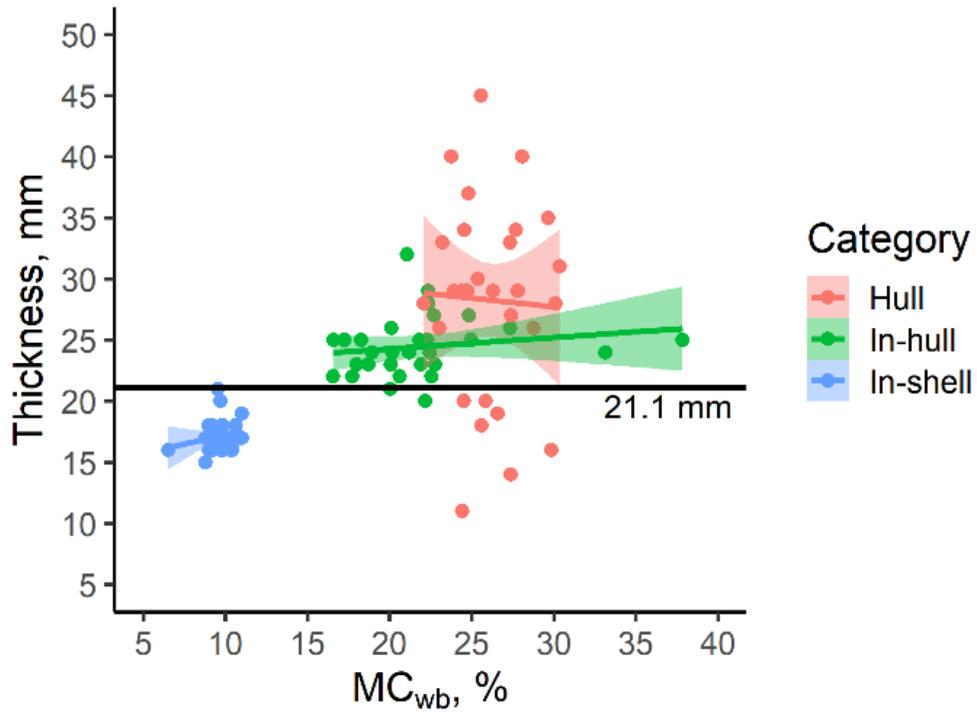
Figure AC.5 Separation of in-shell almonds from hulls and in-hull almonds based on thickness for the Fritz variety
