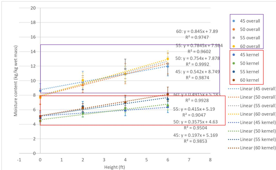
Figure AB.40 Variation of final MC in the overall almonds and almond kernels at different locations in the column dryer with 2.0 m/s air speed (MT)
