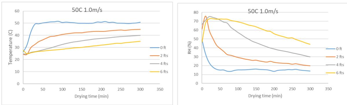
Figure AB.29 Temperature and RH of air in the column drying at 50°C 1 m/s (FR)
