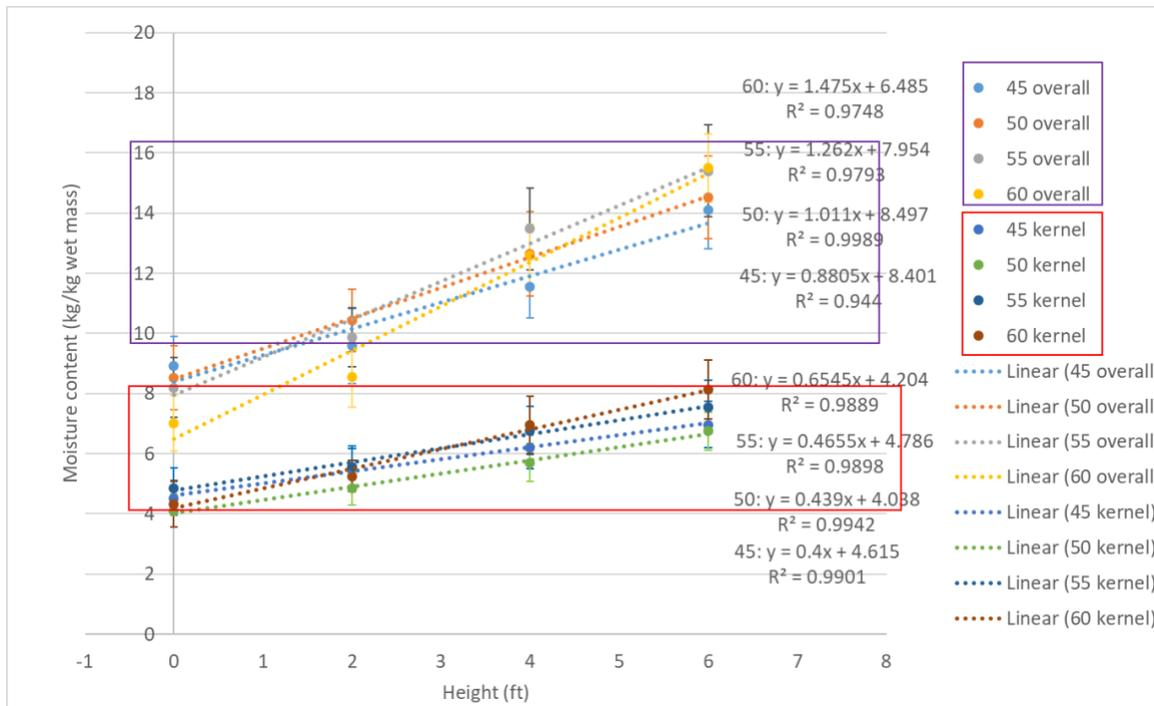
Figure AB.41 Variation of final MC in the overall almonds and almond kernels at different locations in the column dryer with 1.0 m/s air speed (FR)
