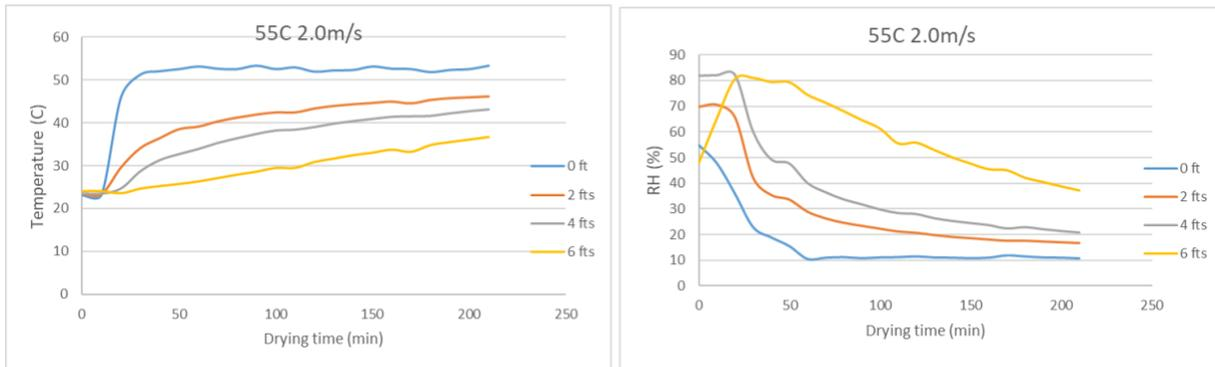
Figure AB.33 Temperature and RH of air in the column drying at 55°C 2 m/s (FR)
