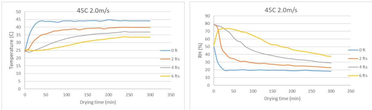
Figure AB.27 Temperature and RH of air in the column drying at 45°C 2 m/s (FR)
