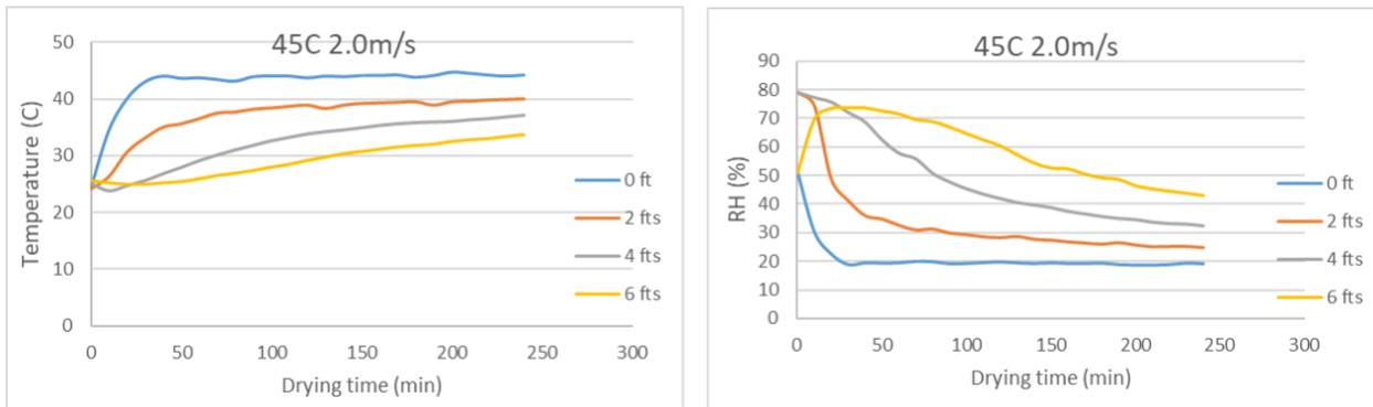
Figure AB.3 Temperature and RH of air in the column drying at 45°C 2 m/s (NP)
