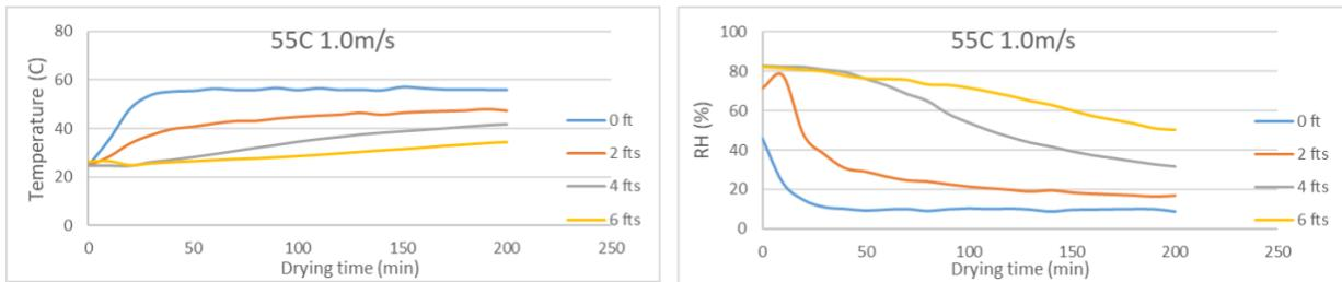
Figure AB.8 Temperature and RH of air in the column drying at 55°C 1 m/s (NP)
