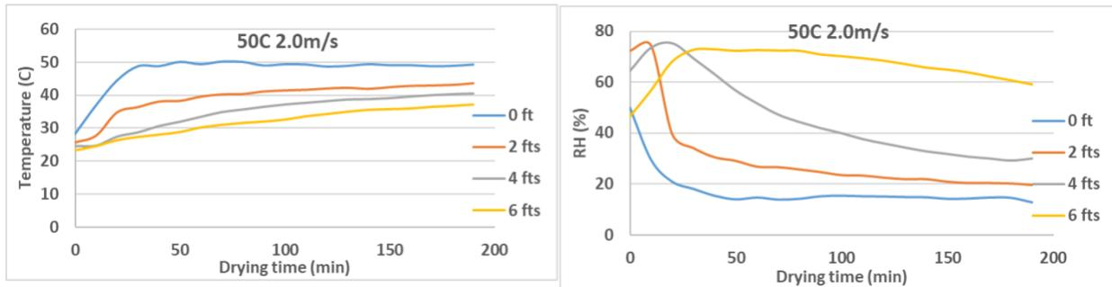
Figure AB.6 Temperature and RH of air in the column drying at 50°C 2 m/s (NP)
