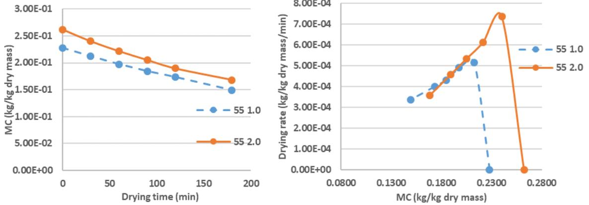
Figure AB.7 Moisture content and drying rate of column drying at 55°C (NP)
