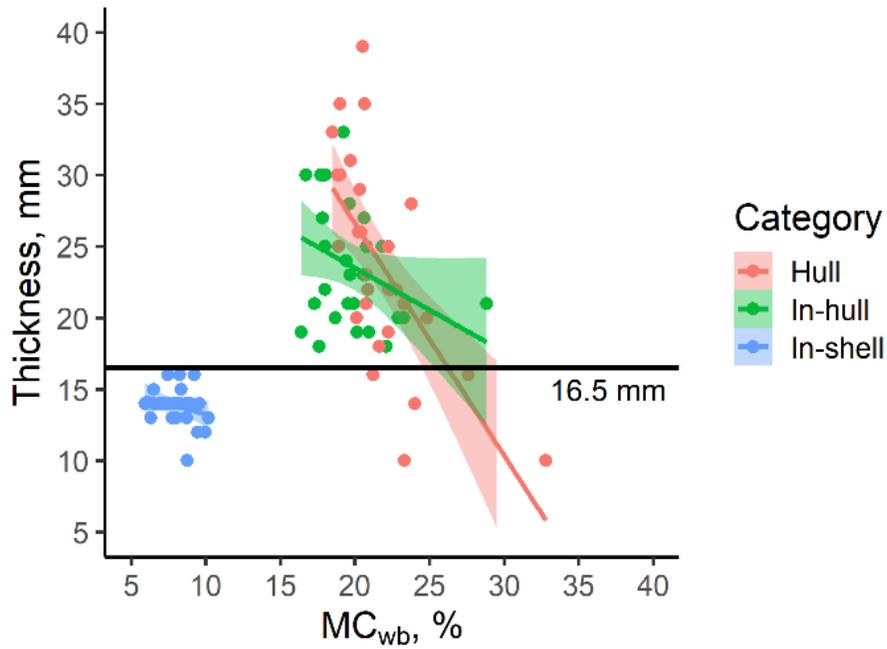
Figure AC.1 Separation of in-shell almonds from hulls and in-hull almonds based on thickness for the Nonpareil variety
