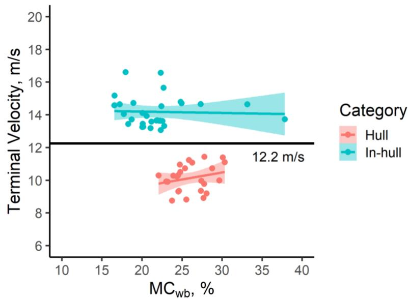
Figure AC.6 Separation of hulls and in-hull almonds based on terminal velocity for the Fritz variety
