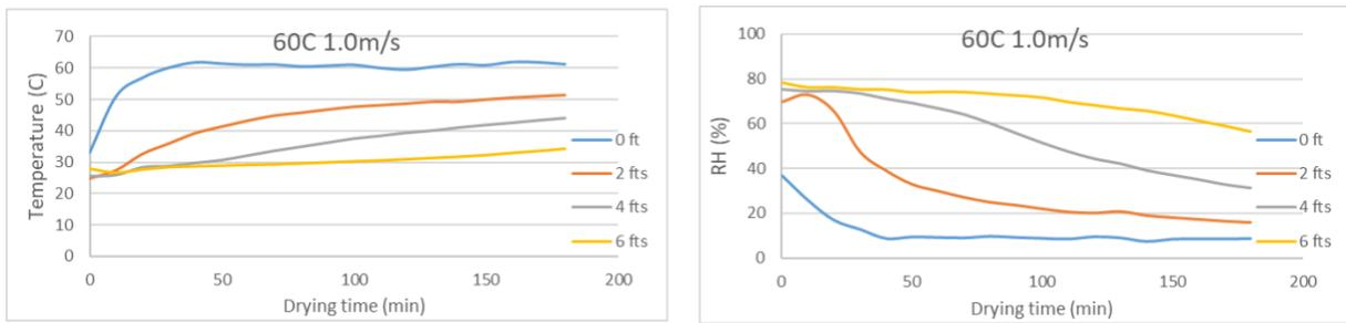
Figure AB.11 Temperature and RH of air in the column drying at 60°C 1 m/s (NP)
