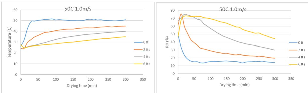
Figure AB.17 Temperature and RH of air in the column drying at 50°C 1 m/s (MT)
