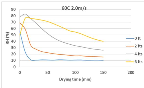
Figure AB.24 Temperature and RH of air in the column drying at 60°C 2 m/s (MT)
