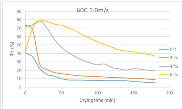
Figure AB.35 Temperature and RH of air in the column drying at 60°C 1 m/s (FR)
