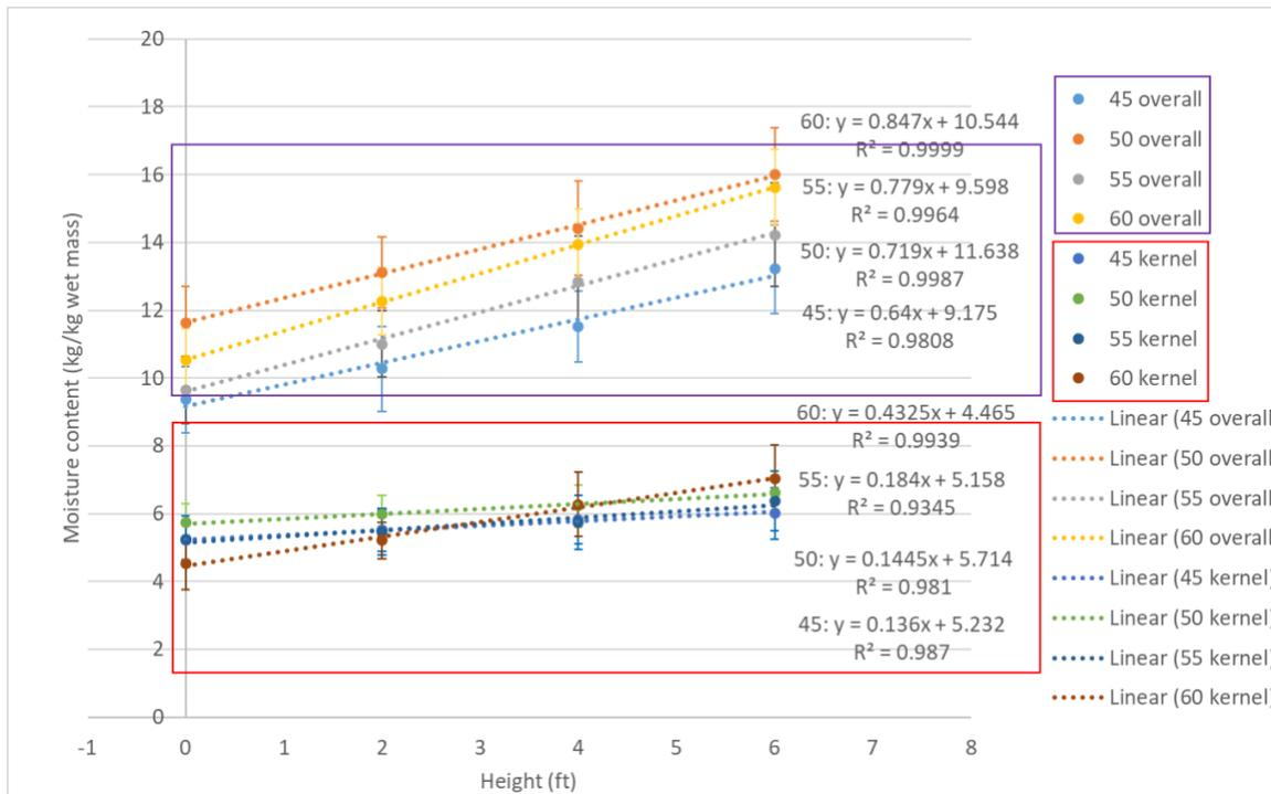
Figure AB.37 Variation of final MC in the overall almonds and almond kernels at different locations in the column dryer with 1.0 m/s air speed (NP)
