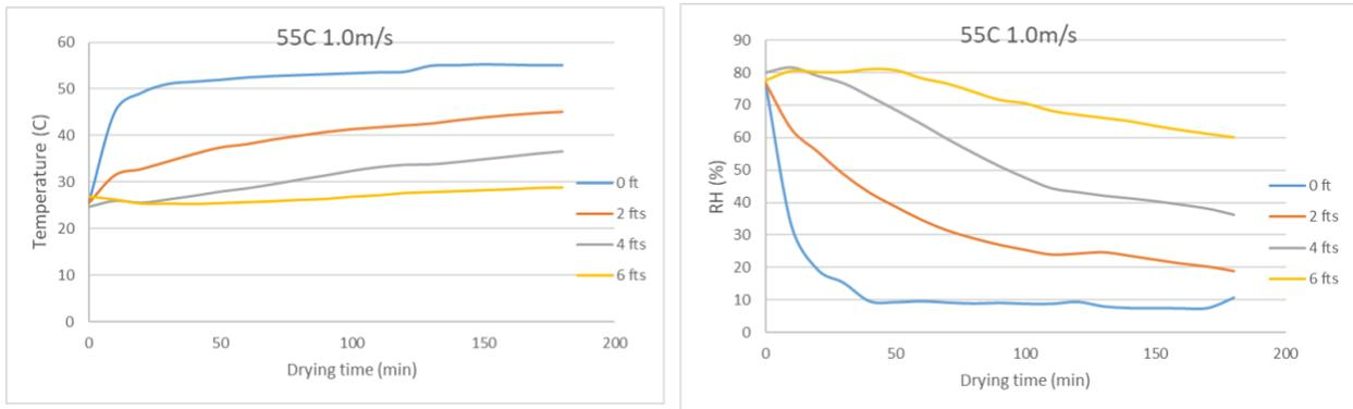
Figure AB.20 Temperature and RH of air in the column drying at 55°C 1 m/s (MT)
