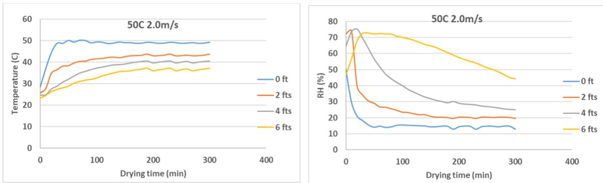
Figure AB.30 Temperature and RH of air in the column drying at 50°C 2 m/s (FR)
