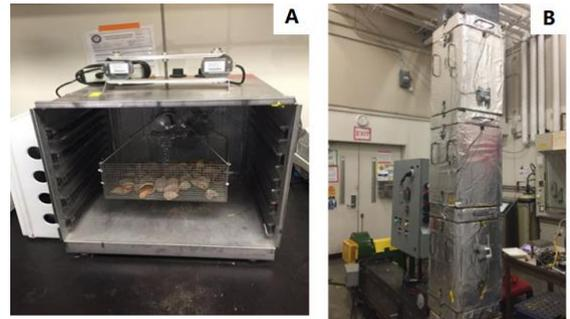
Figure E.2 A) Benchtop dryer and B) Column dryer
