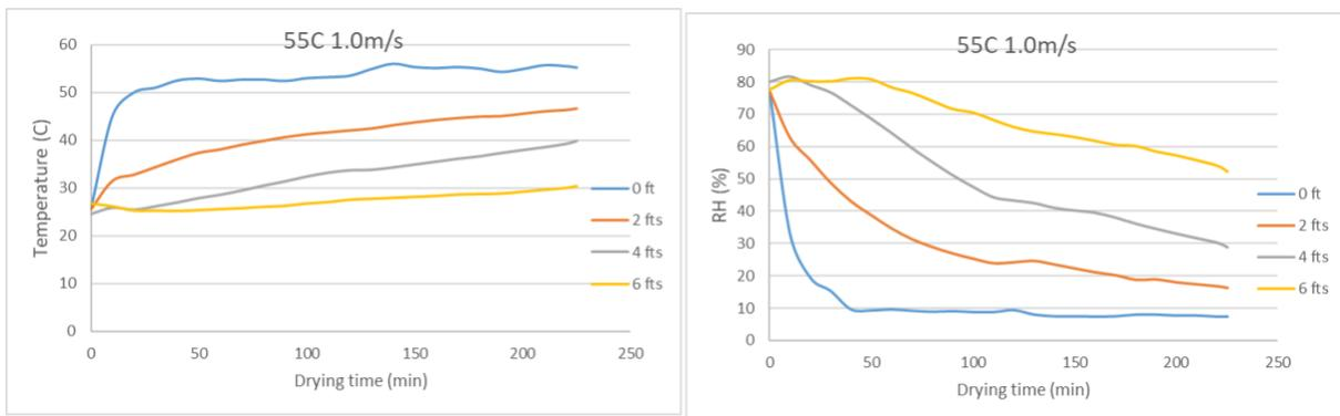
Figure AB.32 Temperature and RH of air in the column drying at 55°C 1 m/s (FR)
