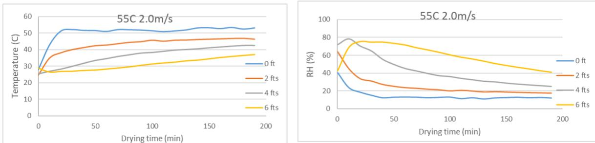
Figure AB.9 Temperature and RH of air in the column drying at 55°C 2 m/s (NP)
