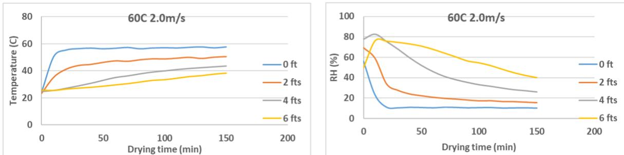
Figure AB.12 Temperature and RH of air in the column drying at 60°C 2 m/s (NP)
