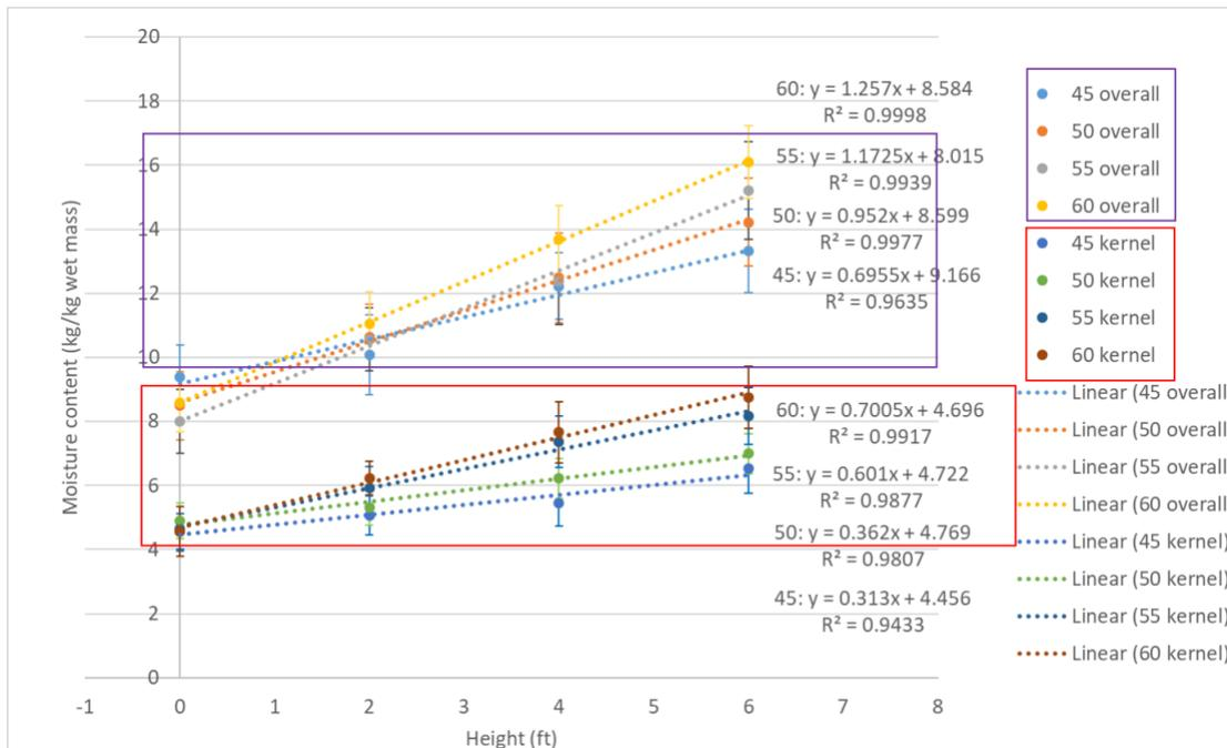
Figure AB.42 Variation of final MC in the overall almonds and almond kernels at different locations in the column dryer with 2.0 m/s air speed (FR)
