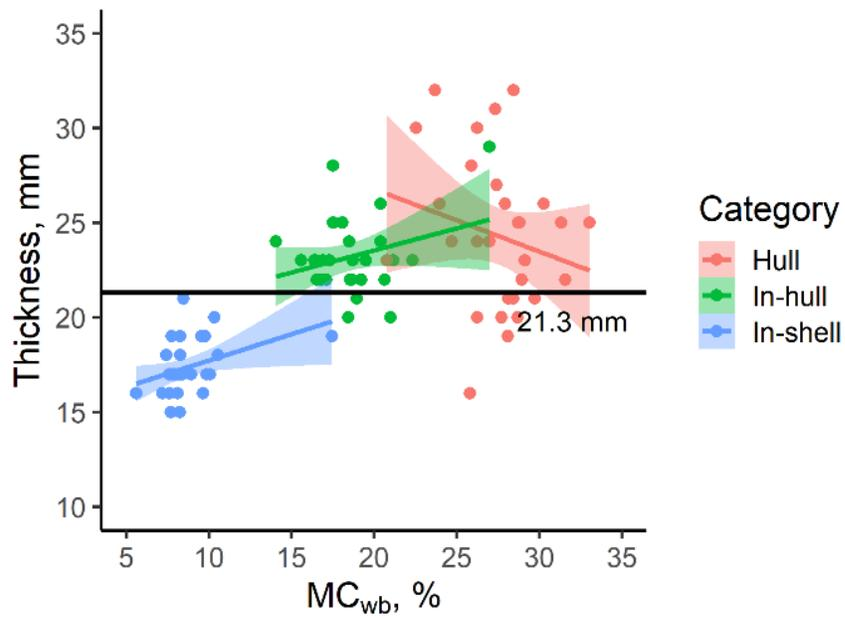
Figure AC.3 Separation of in-shell almonds from hulls and in-hull almonds based on thickness for the Monterey variety
