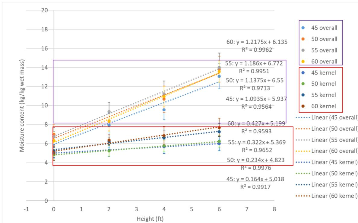
Figure AB.39 Variation of final MC in the overall almonds and almond kernels at different locations in the column dryer with 1.0 m/s air speed (MT)
