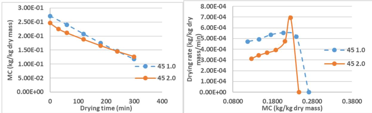
Figure AB.25 Moisture content and drying rate of column drying at 45°C (FR)
