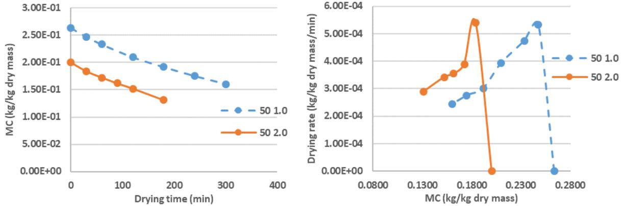
Figure AB.4 Moisture content and drying rate of column drying at 50°C (NP)
