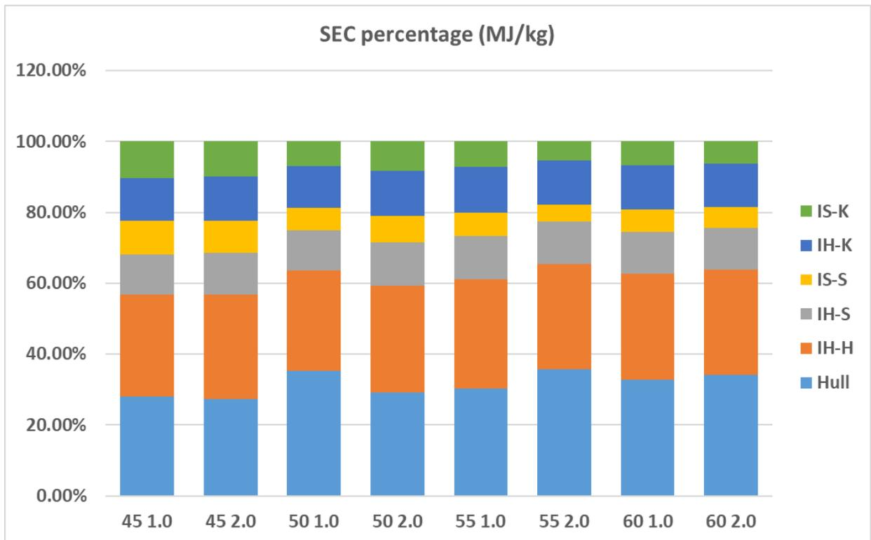
Figure AB.44 Specific energy consumption (SEC) for column dryer at different drying conditions (MT)
