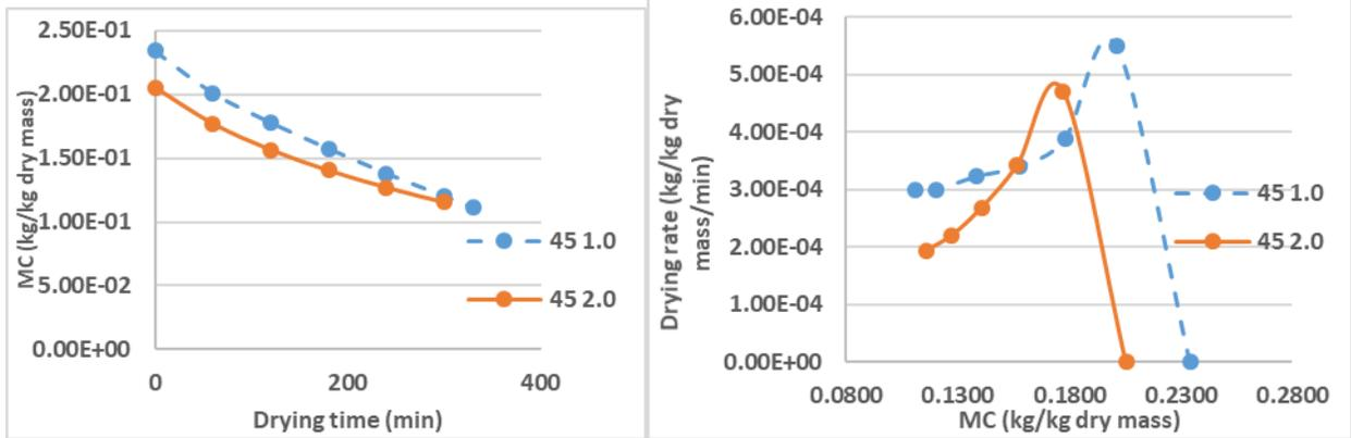
Figure AB.13 Moisture content and drying rate of column drying at 45°C (MT)
