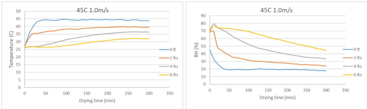
Figure AB.26 Temperature and RH of air in the column drying at 45°C 1 m/s (FR)
