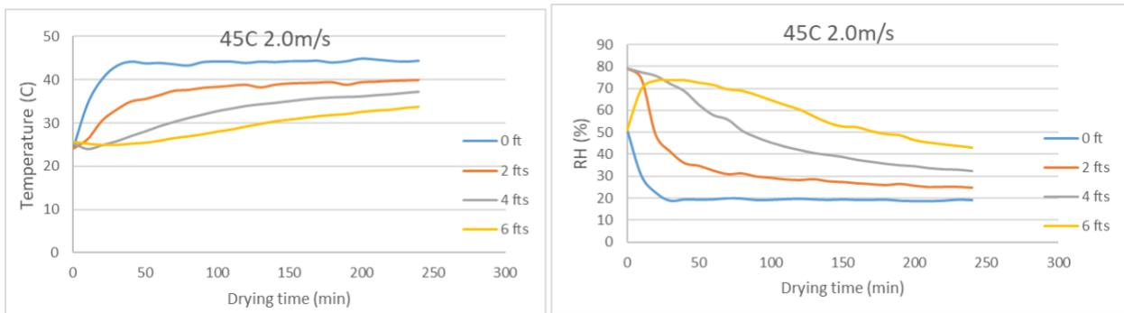
Figure AB.15 Temperature and RH of air in the column drying at 45°C 2 m/s (MT)
