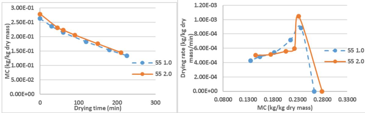
Figure AB.31 Moisture content and drying rate of column drying at 55°C (FR)
