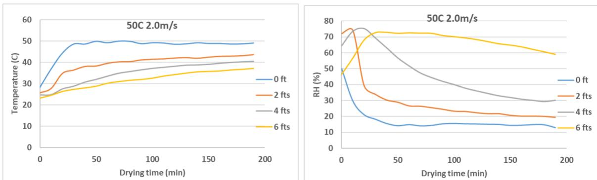
Figure AB.18 Temperature and RH of air in the column drying at 50°C 2 m/s (MT)
