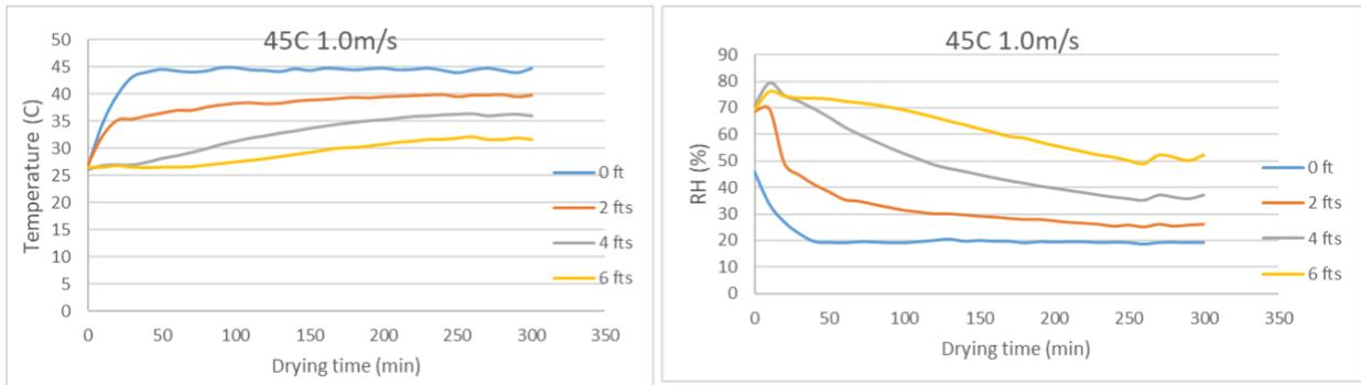
Figure AB.14 Temperature and RH of air in the column drying at 45°C 1 m/s (MT)
