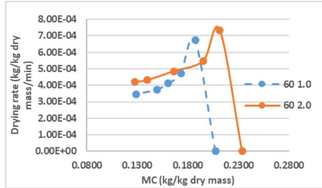
Figure AB.22 Moisture content and drying rate of column drying at 60°C (MT)
