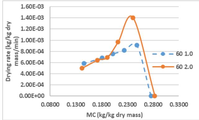
Figure AB.34 Moisture content and drying rate of column drying at 60°C (FR)
