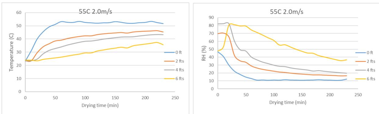
Figure AB.21 Temperature and RH of air in the column drying at 55°C 2 m/s (MT)
