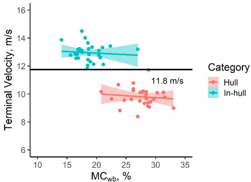
Figure AC.4 Separation of hulls and in-hull almonds based on terminal velocity for the Monterey variety
