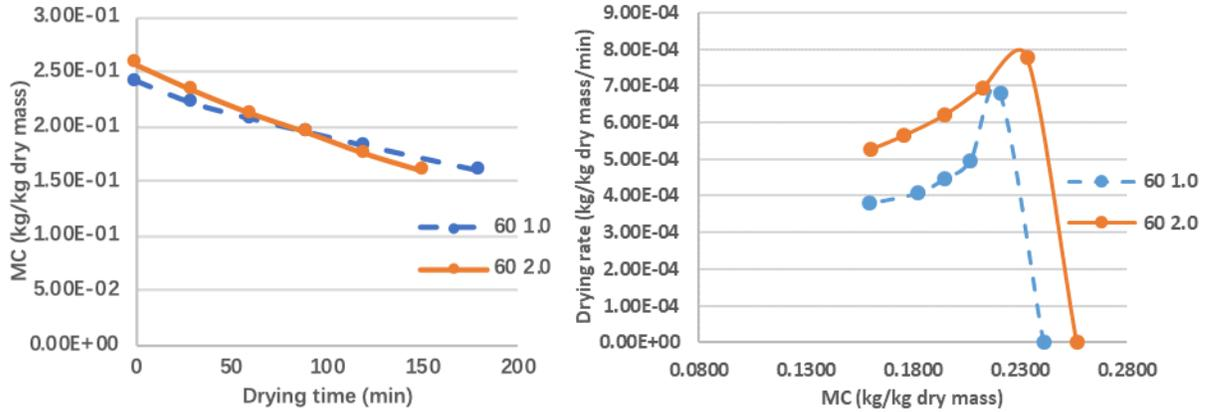
Figure AB.10 Moisture content and drying rate of column drying at 60°C (NP)
