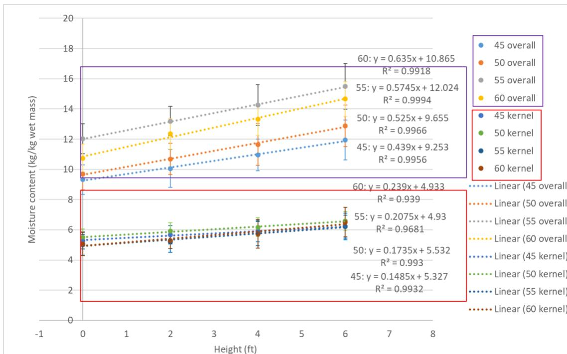
Figure AB.38 Variation of final MC in the overall almonds and almond kernels at different locations in the column dryer with 2.0 m/s air speed (NP)
