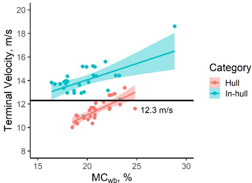
Figure AC.2 Separation of hulls and in-hull almonds based on terminal velocity for the Nonpareil variety
