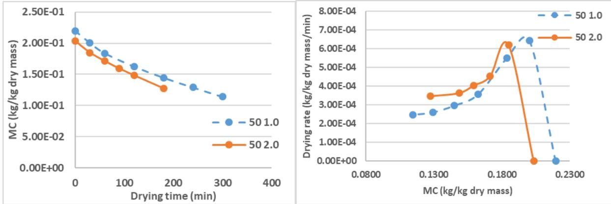
Figure AB.16 Moisture content and drying rate of column drying at 50°C (MT)
