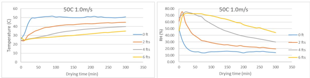
Figure AB.5 Temperature and RH of air in the column drying at 50°C 1 m/s (NP)
