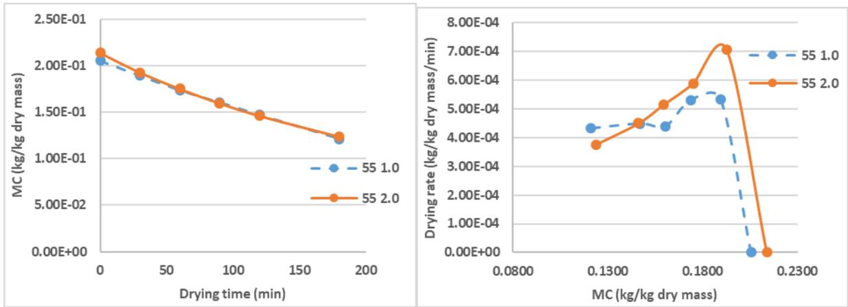
Figure AB.19 Moisture content and drying rate of column drying at 55°C (MT)
