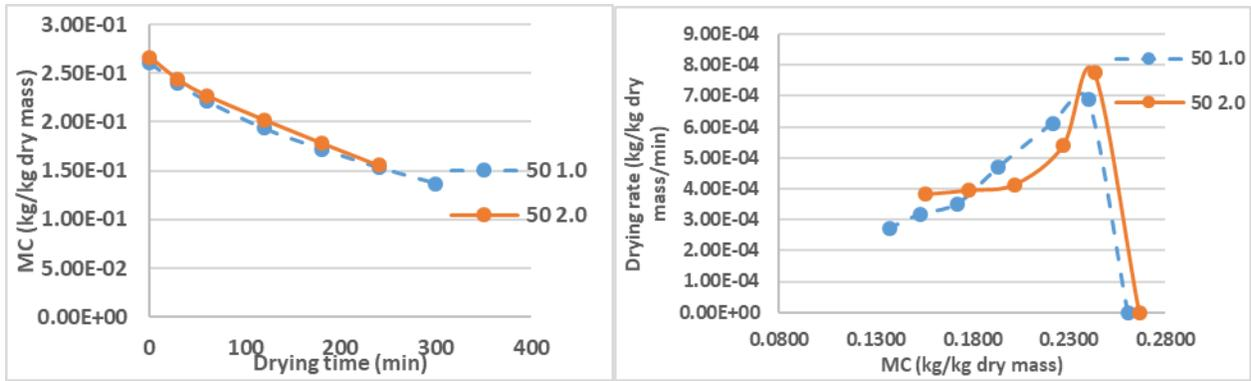
Figure AB.28 Moisture content and drying rate of column drying at 50°C (FR)
