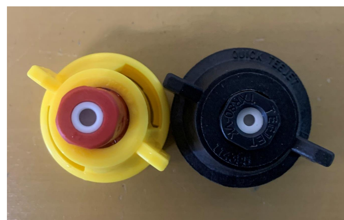
Two nozzles, different exit orifices, same spray flow rate. AITA (04) on the left, TXR (04) on the right. Nozzle on the L makes coarse droplets. The one on the R makes fine droplets.
