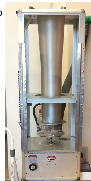
Figure 3. Potter spray tower for application of formulated pesticides to bees at multiples of the maximum application rate
