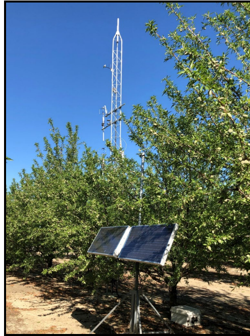
Flux tower in experimental almond orchard containing a mature tree in a weighing lysimeter
