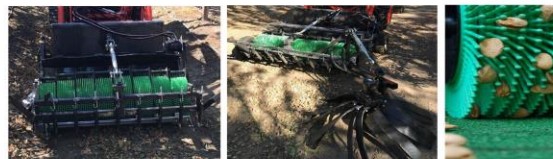
Figure 3. Version 1 of the finger wheel pick-up (left), Version 2 of the finger wheel pickup with side sweeper (middle), close up of how the finger wheel pick up fruit (right).
