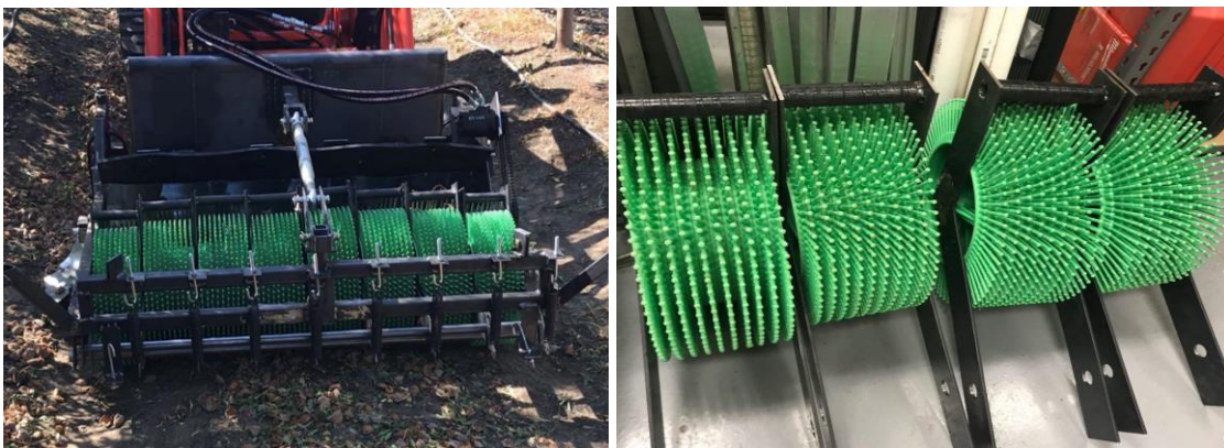
Figure 3. Almond pick up attachment prototype for the California 2019 season.
