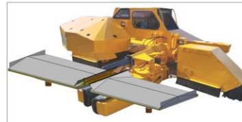
Figure 2. A design rendering of how the screen would look on a side boom shaker (left). Testing a blower where the airflow runs parallel to the ground (right).
