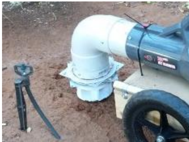
Figure 1. 3D-printed blower head attached to a typical leaf blower using lower velocity air, but adequate to remove leaves and windfall as it moves parallel to the surface, tested in Australia in 2019.
