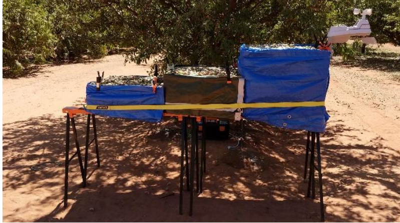
Figure 1. ‘Carmel’ almond fruit stacked into 200-mm, 300-mm and 500-mm drying silos just after shaking. Ambient air can freely enter through the bottom of the silo. Tested at Century Orchards in the 2019 Australian season.
