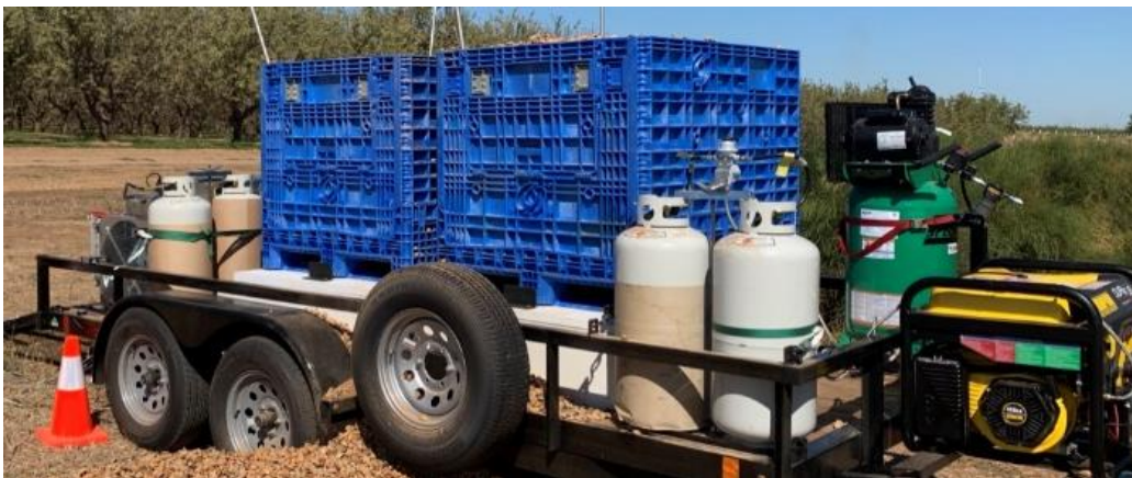
Figure 5. In-field bin batch dryer at Nickels soil lab, California, 2019 season.
