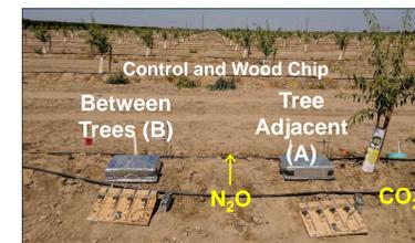
Fig. 4 static flux chambers have three locations: adjacent (A) and between trees (B), and in the alleyway.
