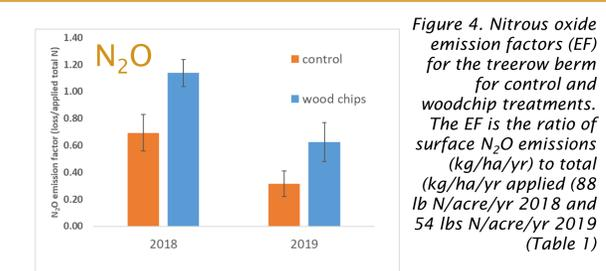
Figure 4. Nitrous oxide emission factors (EF) for the treerow berm for control and woodchip treatments. The EF is the ratio of surface N<sub>2</sub>O emissions (kg/ha/yr) to total (kg/ha/yr applied (88 lb N/acre/yr 2018 and 54 lbs N/acre/yr 2019 (Table 1)
